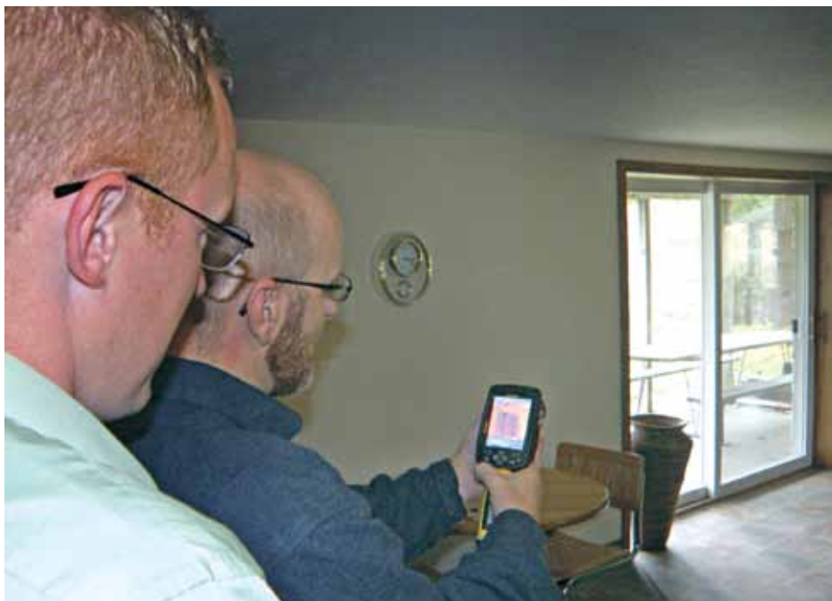
Matt Rosendaul (front) demonstrates how an infrared camera can locate cold spots. Below, he shows me how a blower door test is set up.
