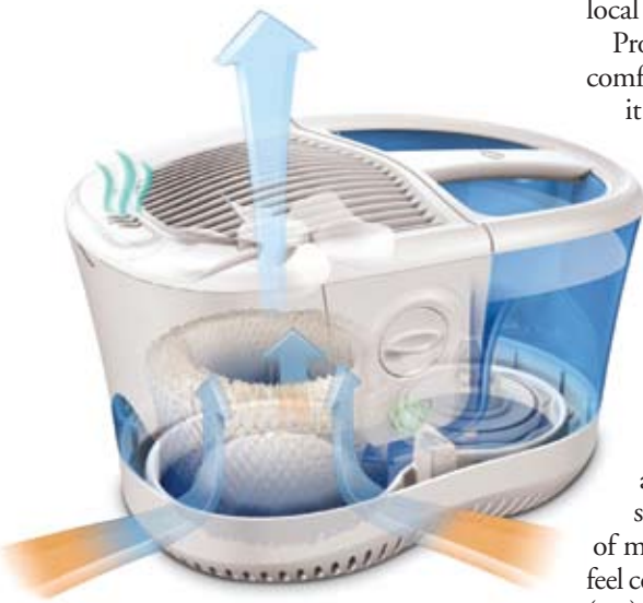
The room air flows through a wet wick inside this evaporative humidifier to add moisture to the air.
