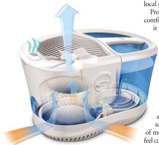
The room air flows through a wet wick inside this evaporative humidifier to add moisture to the air.
