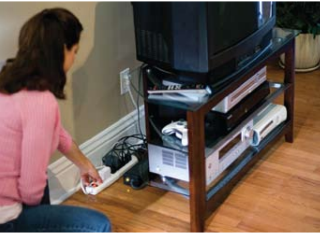
Power strips are an easy way to turn power off to several items without unplugging devices one by one.
