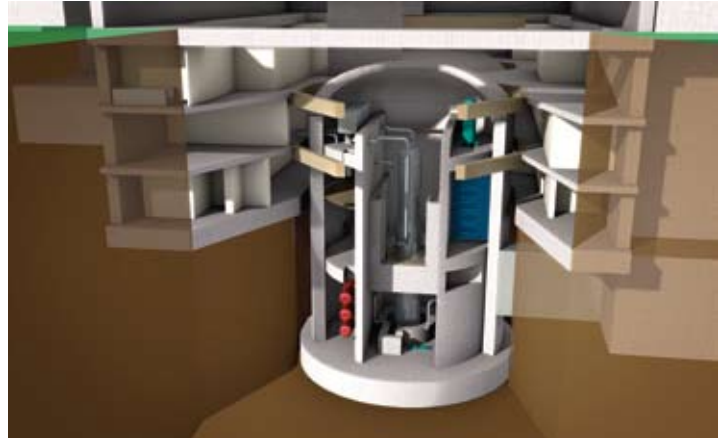
Conceptual drawing of a single B&W mPower nuclear reactor module inside its own independent, underground containment.
