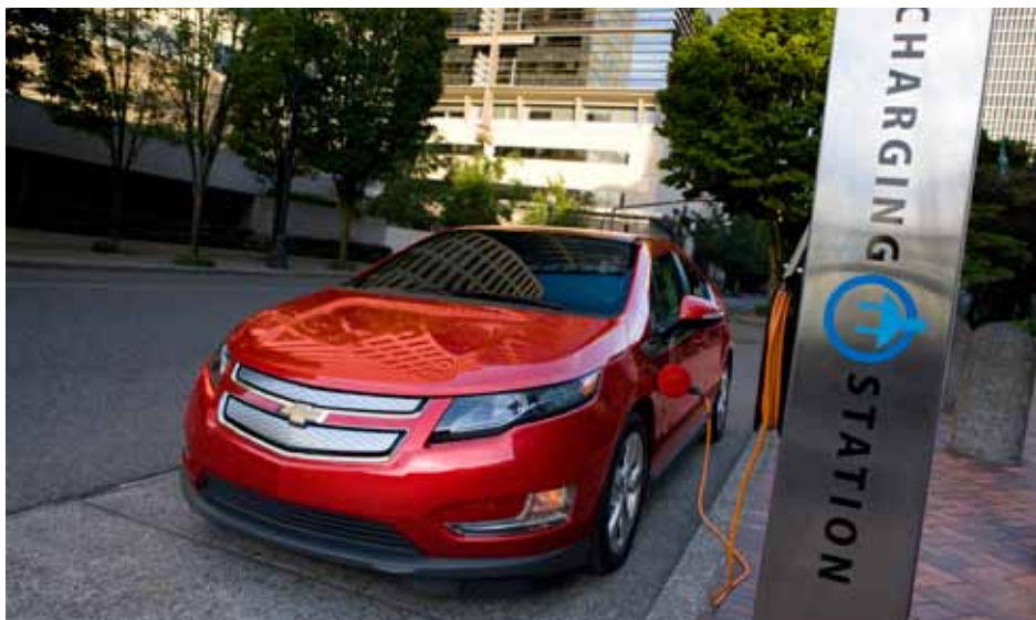
Charging stations provide a dedicated 240-volt circuit, similar to that used for electric clothes dryers. Using this type of a station, the all-electric Nissan Leaf can be charged in four hours while the 2011 Chevy Volt, pictured, can be ready to hit the highway in as little as three hours.
