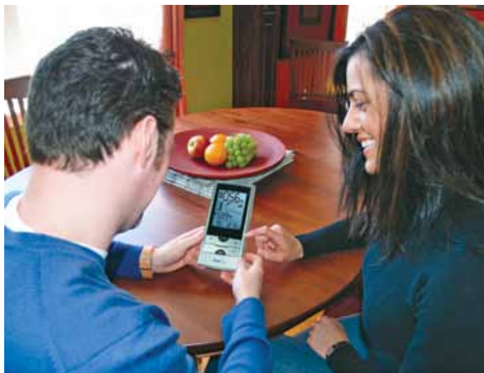
In-home displays like the PowerCost Monitor™ are being developed to provide a variety of information related to energy use, including how many kilowatt hours you have consumed and how much money you are currently spending on electricity.
