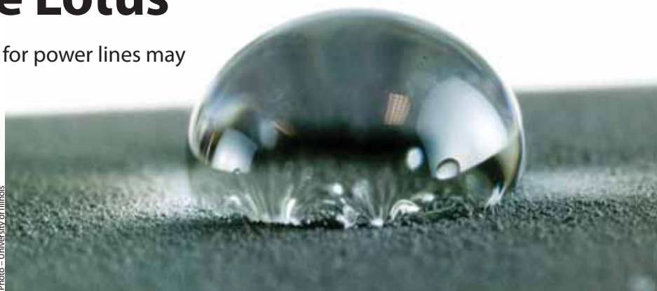
Surfaces coated with a superhydrophobic spray make them virtually “unwetterable.” That means coated power lines would repel freezing rain, preventing damaging ice from forming.
