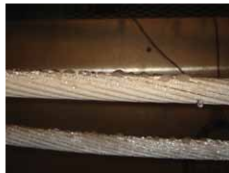
Lines treated with a superhydrophobic coating repel liquids and prevent major ice accumulation. Any ice that might sit on the lines would be easily blown off by wind or vibration from the power flow.
