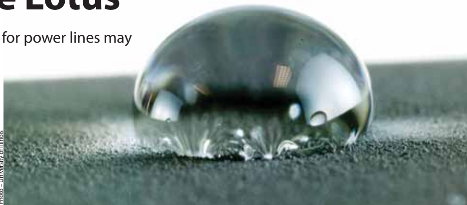
Surfaces coated with a superhydrophobic spray make them virtually “unwettable.” That means coated power lines would repel freezing rain, preventing damaging ice from forming.
