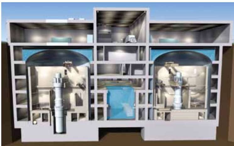
Conceptual drawing of an underground containment structure housing two Babcock & Wilcox mPower reactor modules.
