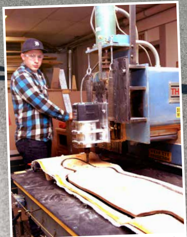
Besides skis, Shaggy's has started making longboards (skateboards). Here, Jeff Thompson mills out the shape of a longboard deck.
