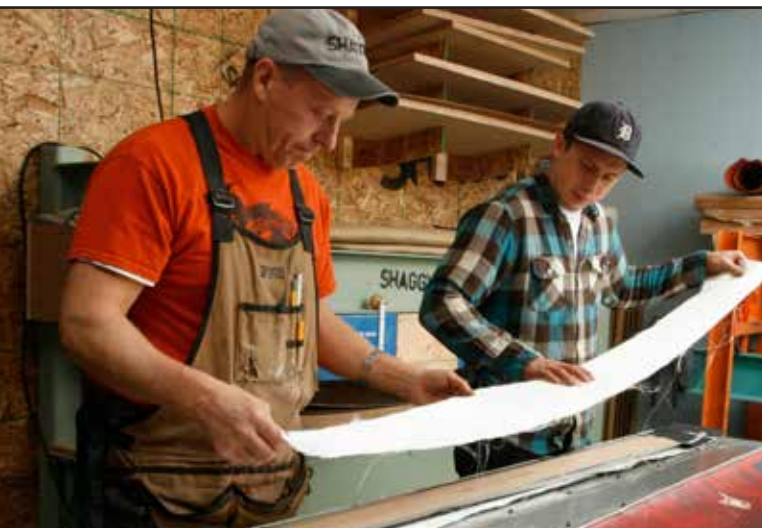
John (L) and Jeff Thompson, of Shaggy's Copper Country Skis, prepare materials that will be pressed into skis, including an ash wood core, Durasurf 4001 base, triaxial fiberglass, damping rubber strips, steel edges, ABS sidewalls, Durasurf tip/tail spacer, and a graphic topsheet.
