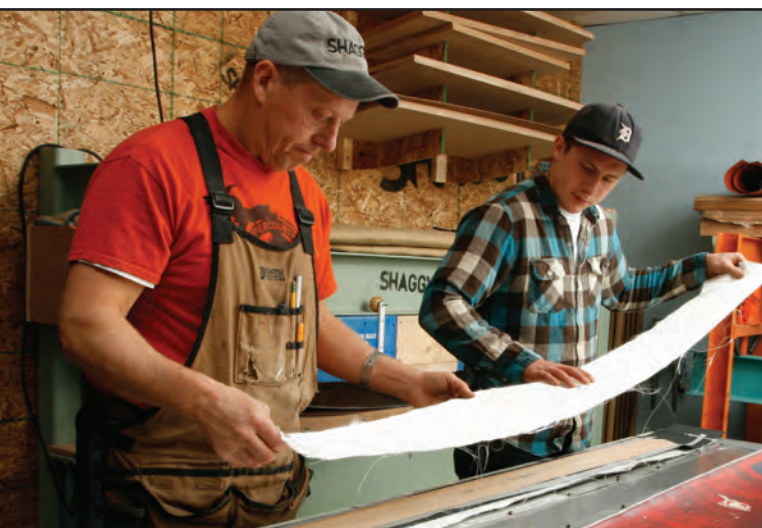
John (L) and Jeff Thompson, of Shaggy's Copper Country Skis, prepare materials that will be pressed into skis, including an ash wood core, Durasurf 4001 base, triaxial fiber glass, damping rubber strips, steel edges, ABS sidewalls, Durasurf tip/tail spacer, and a graphic topsheet.
