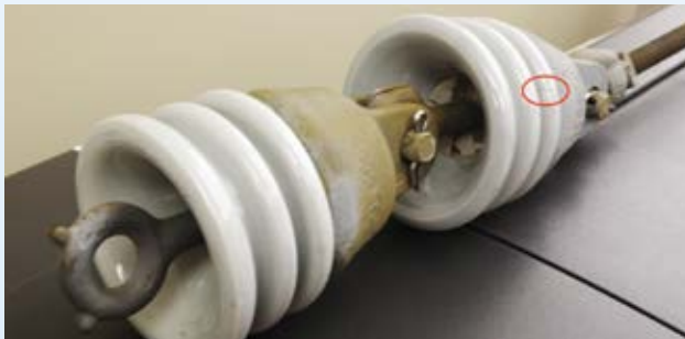
This set of insulating bells has a tiny crack (see circle) that let moisture in, leading to an arc and pole fire.
